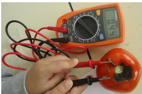
Figure 13 - Measurement of p.d. and current intensity of biological batteries. Calculation of the maximum power supplied.
