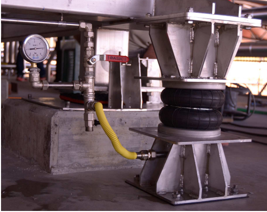
Figure 9: Example of CDM air cushion mounted on the equipment.
