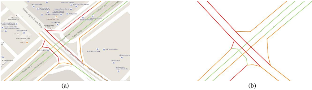
Fig. 7. (a) Images of unprocessed HTML file (b) Images of processed and clutter removed HTML file
