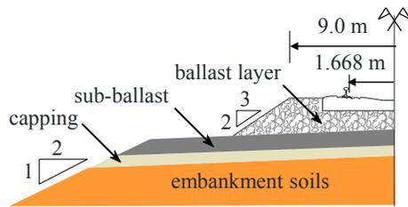
**Figure 2:** Schematic track cross-section (after Paixão, 2014).
