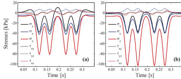
Figure 7: Time history of stresses in element A for the train at 220 km/h: (a) linear ballast; (b) nonlinear ballast.
