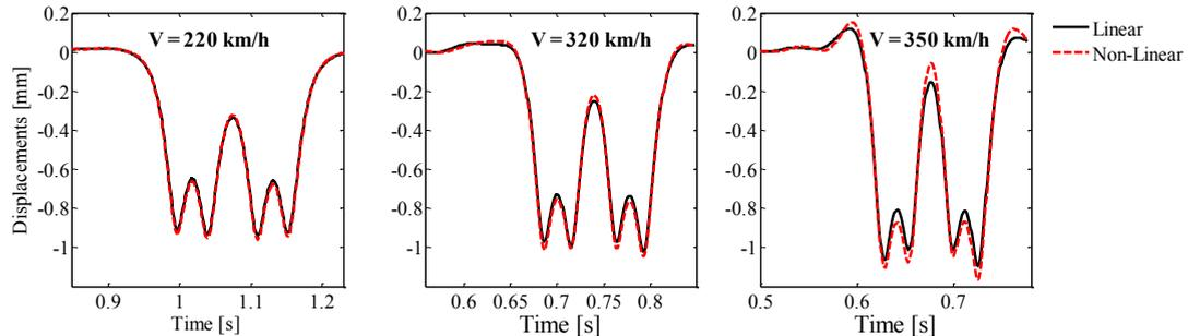
**Figure 5:** Time history of dynamic rail displacements at different speeds, obtained considering the linear-elastic behaviour of ballast (black lines) and the nonlinear-elastic behaviour of ballast (red lines).
