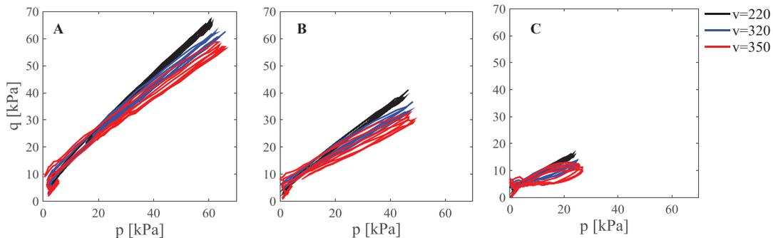
Figure 10: Stress paths p-q, in elements A, B and C, for the passage of the train at several speeds.
