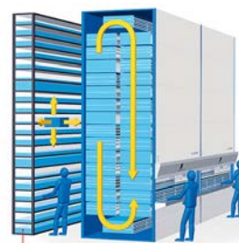
Fig. 2. Comparison between a motionless storage system and a vertical carousel storage unit [7]
