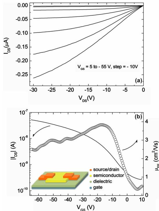
FIG. 5. (Color online) (a) Output characteristics ( $I_{DS}$ - $V_{DS}$ ); (b) Transfer characteristics ( $|I_{DS}$ - $V_{GS}$ ) at  $V_D = -5$  V (left axis) and  $\mu_{FE}$  as a function of  $V_{GS}$  (right axis), for a typical  $\text{Cu}_2\text{O}$  TFT produced at RT and annealed in air at 200 °C. The inset shows the structure of the bottom gate TFT.
