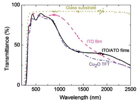
FIG. 4. (Color online) Optical transmission spectra for the entire  $\text{Cu}_2\text{O}$ -TFT structure including the glass substrate; it is possible to observe that the  $\text{Cu}_2\text{O}$ -TFT is fully transparent to visible light. For comparison purposes, the optical transmission spectra for the glass substrate, the ITO, and the ITO/ATO films are also presented.
