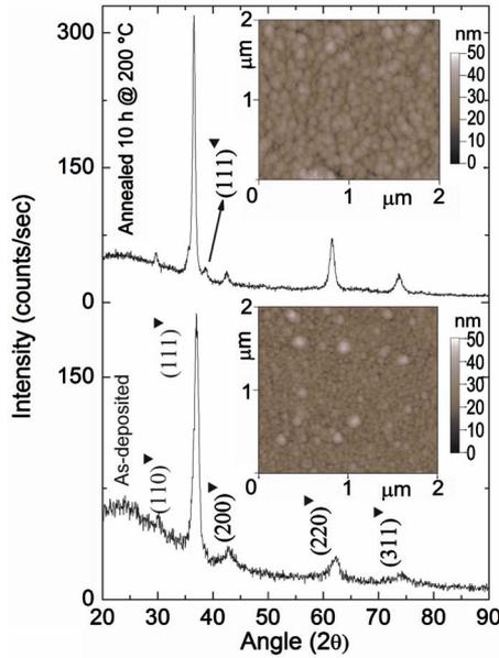
FIG. 2. (Color online) X-ray pattern of the  $\text{Cu}_2\text{O}$  film annealed at  $200^\circ\text{C}$  in air for 10 h in comparison with the as-deposited film. (Symbol representations:  $\blacktriangledown$ — $\text{Cu}_2\text{O}$  phase and  $\blacktriangleleft$ — $\text{CuO}$  phase.) The insets show the AFM images of the corresponding films.
