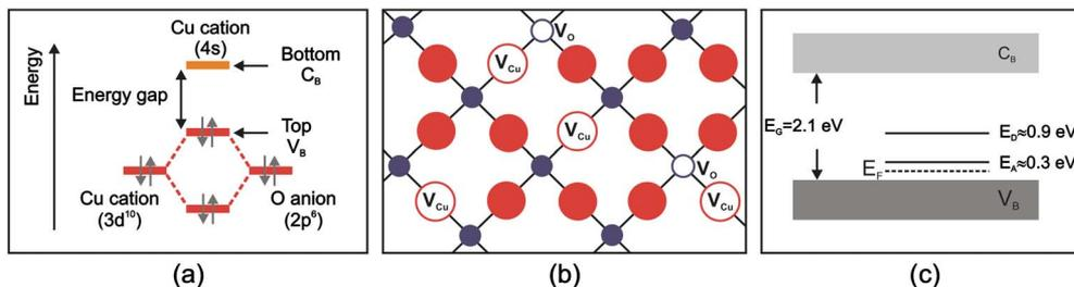
FIG. 1. (Color online) (a) Chemical bond between an oxide ion and a cation that has a closed-shell electronic configuration; (b) a pictorial representation of the more important defects in Cu<sub>2</sub>O; and (c) a simple electronic model proposed by Brattain, with a compensated semiconductor with one acceptor level at 0.3 eV and a deep donor level at 0.9 eV from  $V_B$ .
