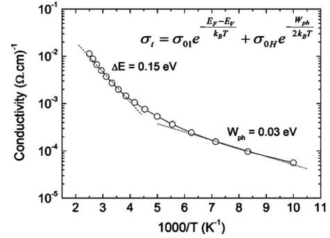
FIG. 3. Temperature dependence of dark conductivity for a  $\text{Cu}_2\text{O}$  thin film with 270 nm. The equation represents the conduction mechanisms for this type of semiconductors. For higher temperatures the conductivity is controlled by an acceptor center located 0.3 eV above the top of  $V_B$  ( $V_{\text{Cu}}$ ) while for low temperatures the conductivity is controlled by hopping.
