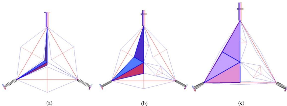
**Figure 2.** Three configuration of screen and underlying assemblage of D-bars: at  $t = 0$  s (a),  $t = 25$  s (b), and  $t = 50$  s (c). The boundary springs and the actuator ram are represented with amplified scales.
