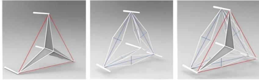
**Figure 1.** (a) TABS configuration; (b) D-bar elements; (c) construction of the WTABS system.
