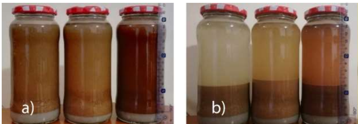
Figure 4. Expedited sedimentation test: a) start of the test; b) after 50 minutes.
