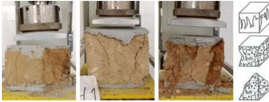
Figure 10. Failure obtained in simple compressed specimens, similar to concrete explosive failure (EN 12390-3, 2019)
