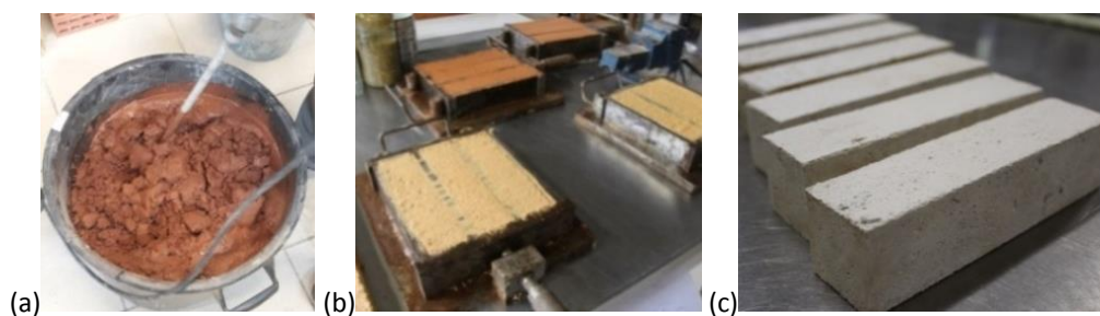
Figure 2. Production of the T_E mortar (a), prismatic specimens of T_AP and T+CL in the metallic moulds (b) and prismatic specimens of C mortar (c).
