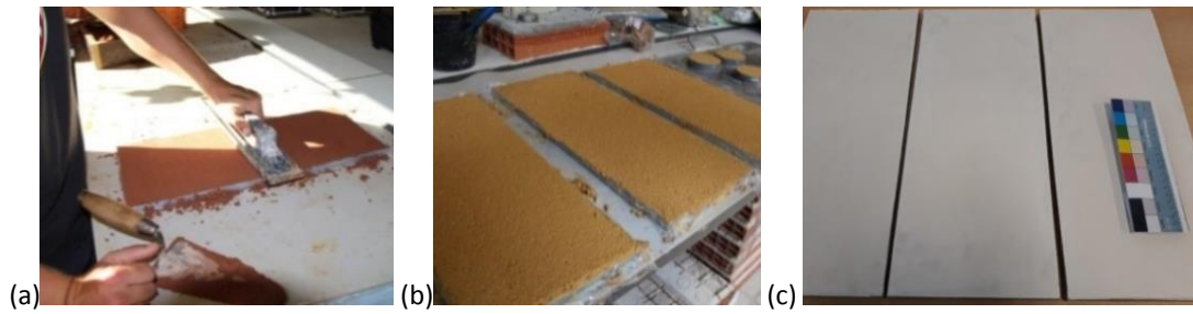
Figure 3. Finishing of planar specimen of T AP plaster (a) and planar specimens of T+CL plaster (b) and planar specimens of G plaster (c).
