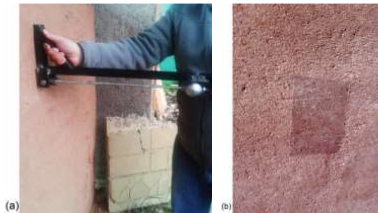
Fig. 4 Sphere impact (a) and surface cohesion (b) tests on a plaster
