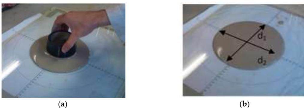
**Figure 7.** Slump test, (a) Lift the cone; (b) Spread sample at stoppage.
