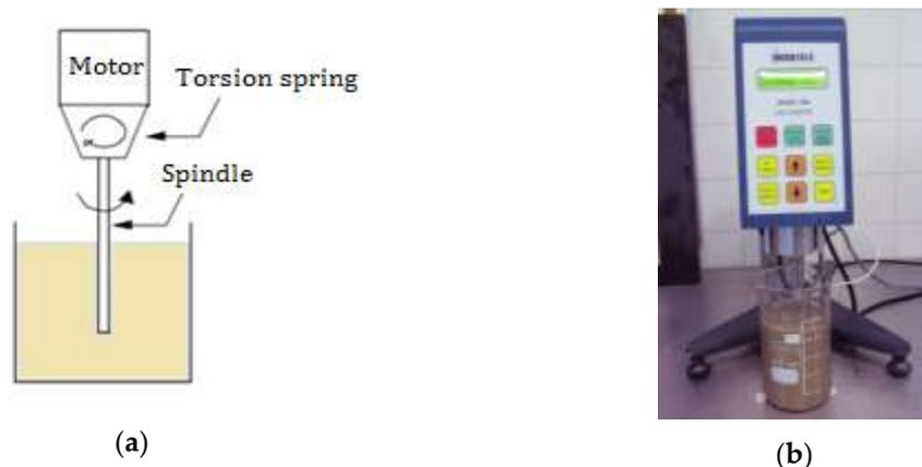
**Figure 4.** Viscometer: (a) Schematic diagram of a Brookfield-type viscometer; (b) Brookfield viscometer LV DV-II + PRO with spindle immersed in the sample.
