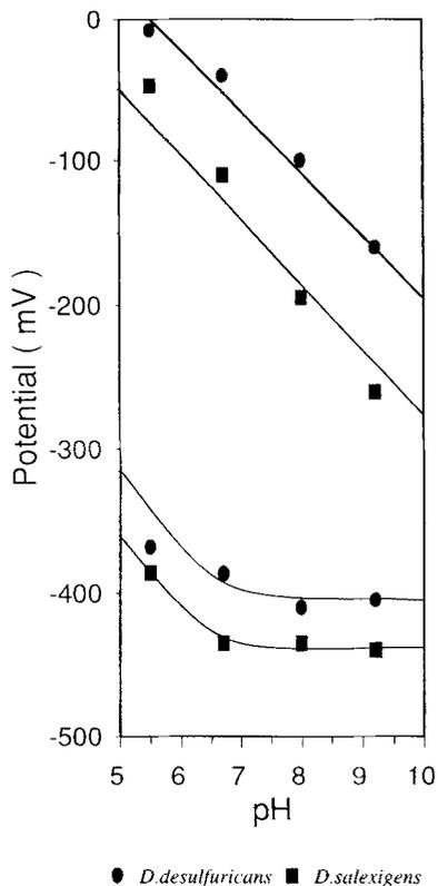
Fig. 3. pH dependence of the oxidation-reduction potentials of *D. desulfuricans* ATCC 27774 (●) and *D. salexigens* (■) flavodoxins. Experimental details as indicated in Materials and Methods.
