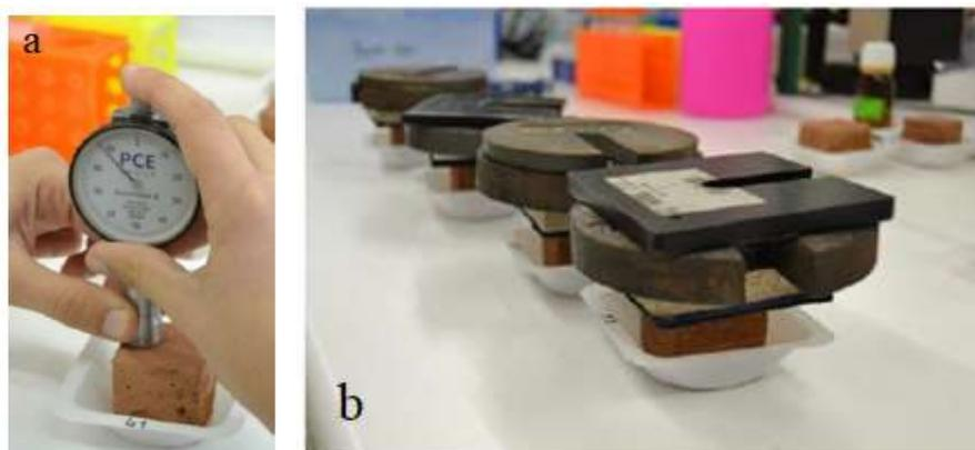
Figure 4. Surface hardness test (a) and surface cohesion test procedure (b).
