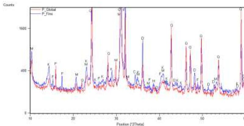
Q – quartz; F – K-feldspar; D – dolomite; M- illite; K – kaolinite; C – calcite; H – hematite.
