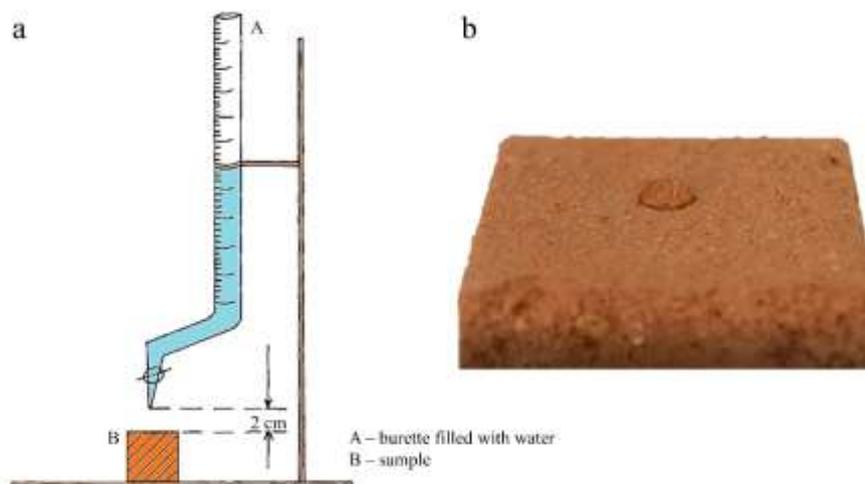
Figure 5. Scheme of the water drop test (a), adapted from RILEM (1980), and drop of water applied on a sample surface, previously treated with a bioproduct, during the water drop test (b).
