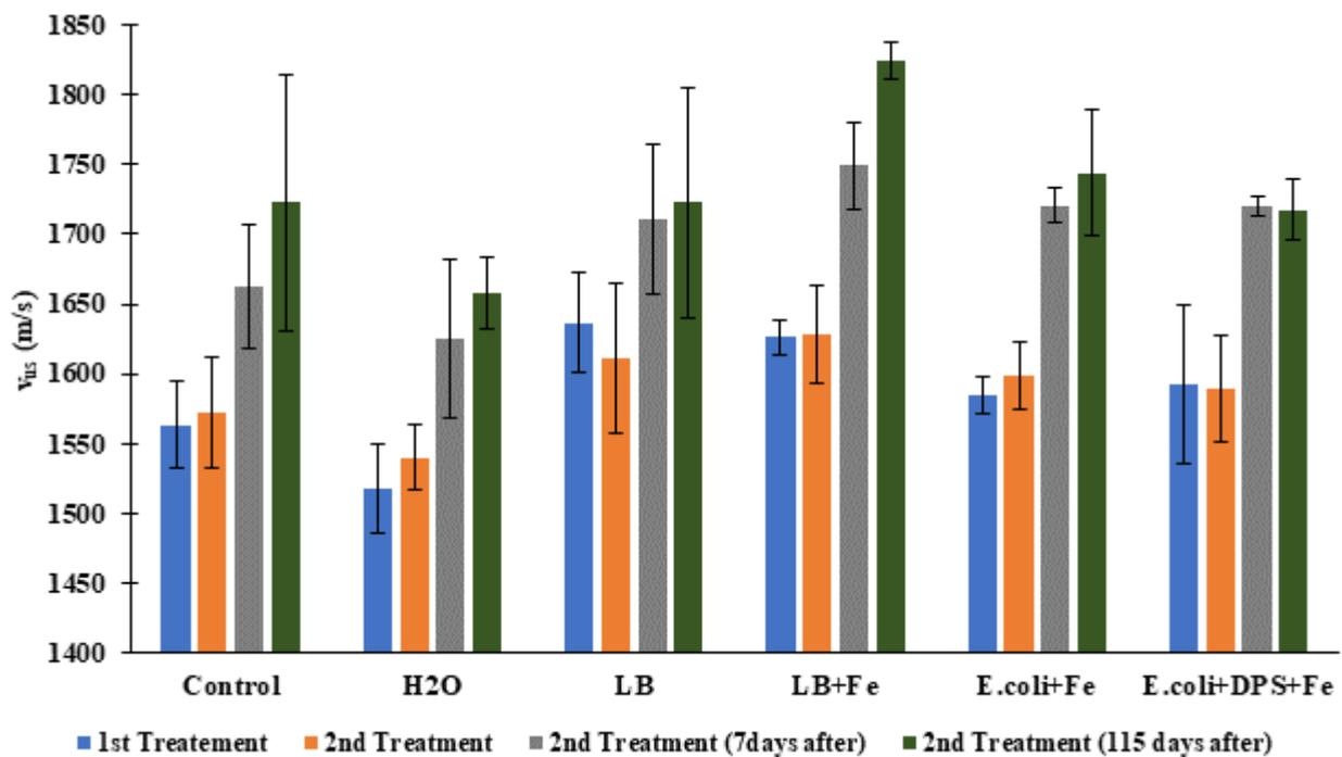
Figure 7. Ultrasound propagation velocity for 1st phase.
