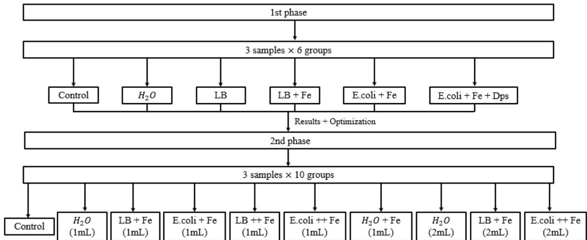
Figure 3. Application scheme of biotreatments to earth-based mortar samples.
