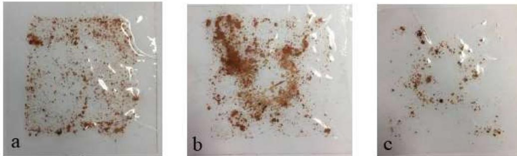
Figure 8. Surface cohesion adhesive tapes from 1st phase: (a) Control; (b) H<sub>2</sub>O and (c) E.coli+Fe.
