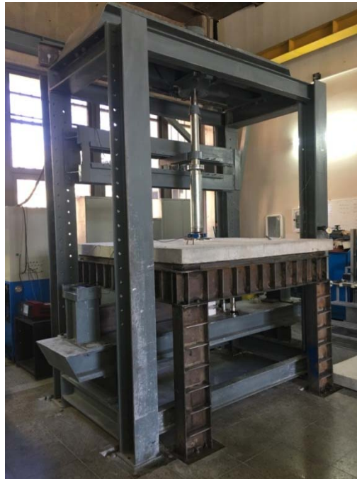
Fig.5. Reaction frame and test setup
