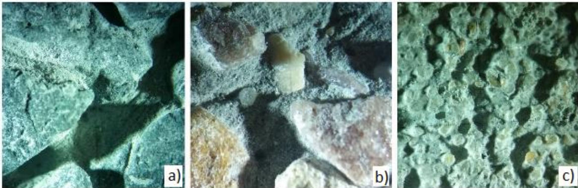
Figure 5 – Exterior surface of samples: (a) BLM washed surface (30x), (b) BLCp washed surface (30x), (c) CM surface (50x)
