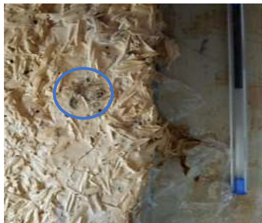
Figure 3. Biological contamination on the RH_30D samples
