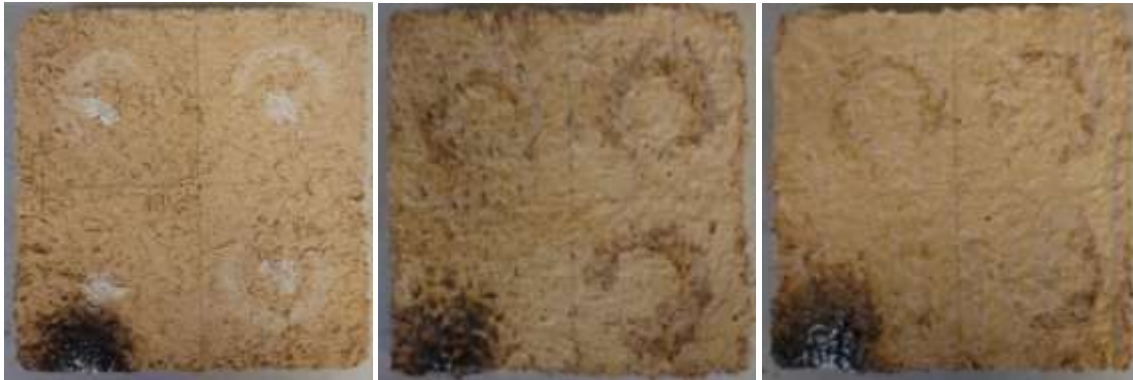
Figure 8. Effect of fire behaviour test (RH_15D- left, RH_30D - centre, RH_30B -right)
