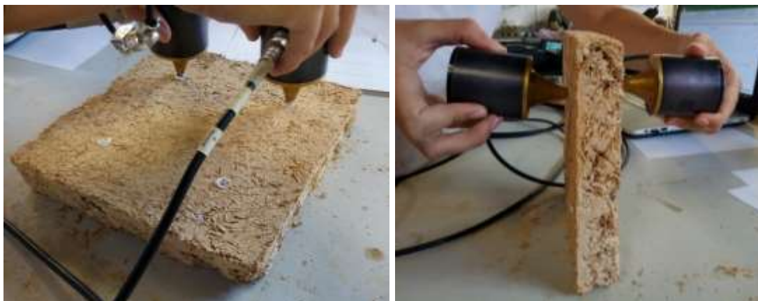
Figure 1. Ultra sound test procedure: (a) Indirect method (b) Direct method.
