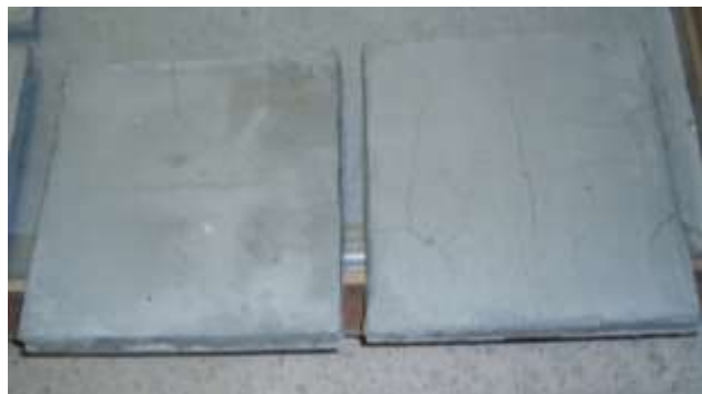
Figure 1 – Restrained shrinkage tests: a) Uniaxial test; b) Slab test
